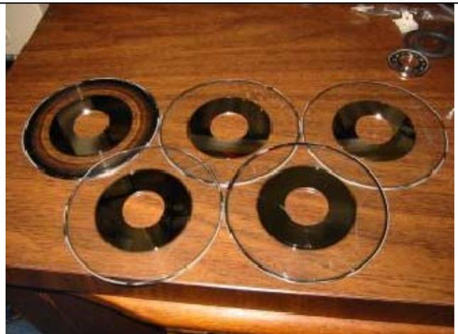
*The damage wasn't limited to just one or two platters. All five of the platters received some level of surface wiping.*
