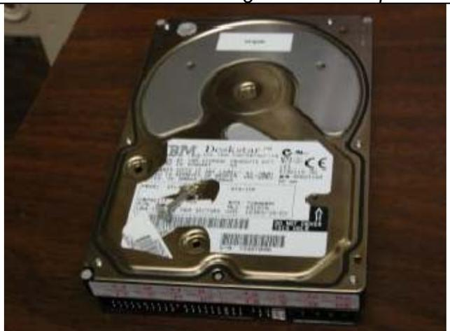
*The first step was to remove the screws on the drive lid. I suspect this voided the warranty, but we were on a mission.*
