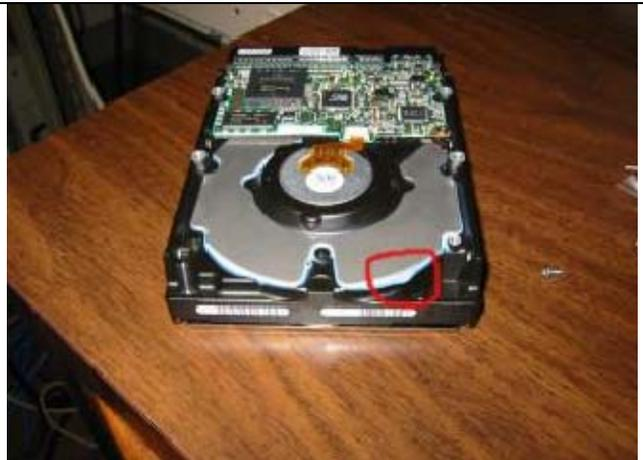
*The first thing I noticed was that a blue ooze had seeped out of the bottom of the drive. At this point I was concerned that some of the goo had possibly oozed into the drive housing and onto the platters.*
